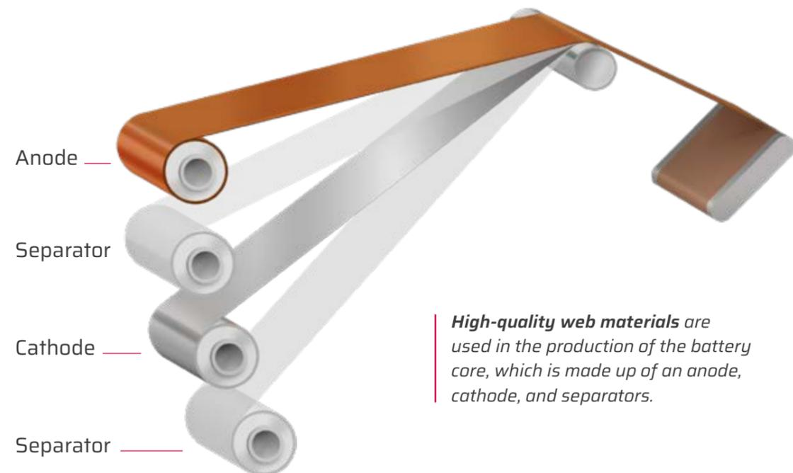
*High-quality web materials are used in the production of the battery core, which is made up of an anode, cathode, and separators.*
